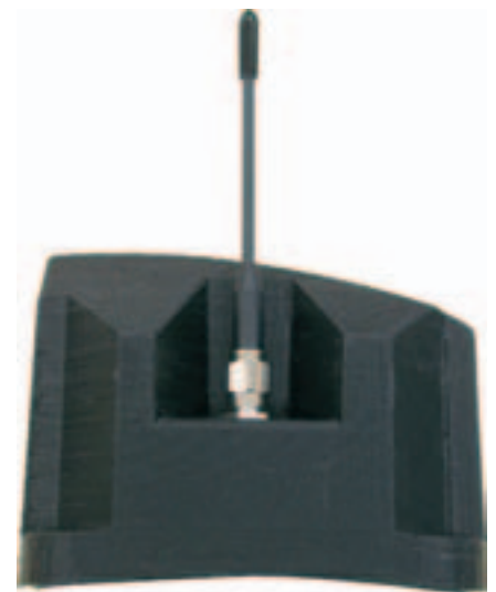
Finished upper part of casing with integrated shock resistant antenna fixation for the enclosing of 868 MHz Ex-radio modules .
